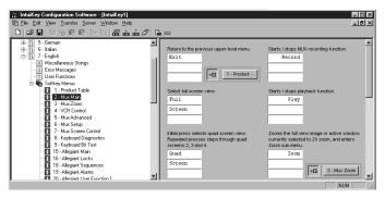
Softkey menu form 1 (1 – **Product Table**) represents the language table's **Product Table** softkey menu which lists all of the devices a keyboard can control. This menu is displayed by a keyboard when its **Prod** keypad button has been pressed.
